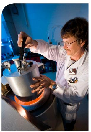
A reactor operator is analyzing a sample of air from the reactor, testing for the presence of fission gases
